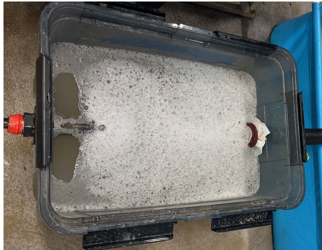
Figure 6. Outlet basin with observed bubbles.
