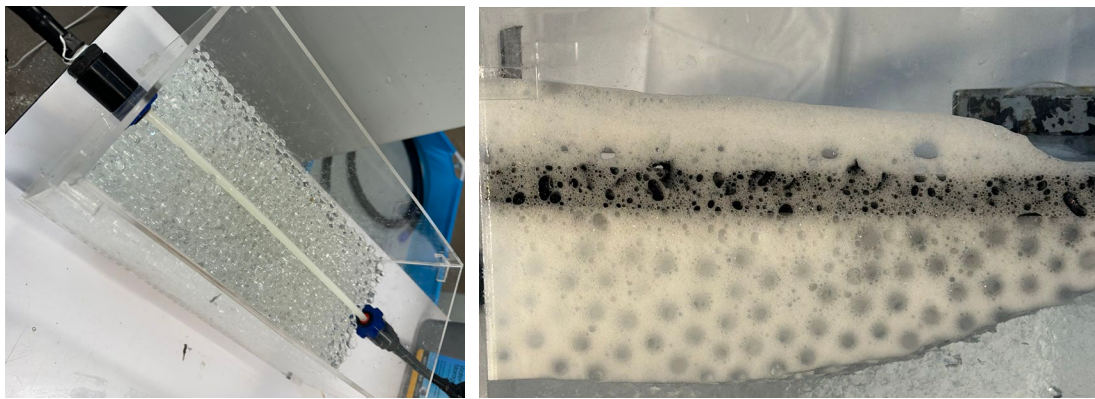
Figure 3. Acrylic box with hydrogels up to the inlet level (left) and dissolving PVA (right).
