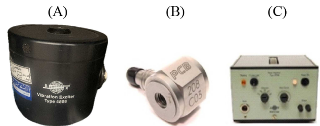
FIGURE 7 | Equipment for conducting the test: (A) Shaker; (B) Force transducer; (C) Amplifier.
