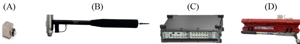
FIGURE 5 | Measurement equipment: (A) Accelerometer; (B) Impact hammer; (C) Pulse data acquisition system; (D) Torque wrench.
