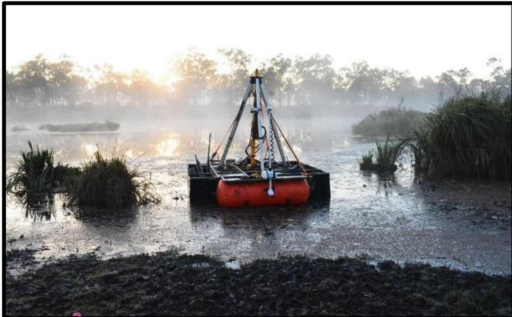
Figure 23: Raft-mounted hydraulic coring rig used in 2018.
