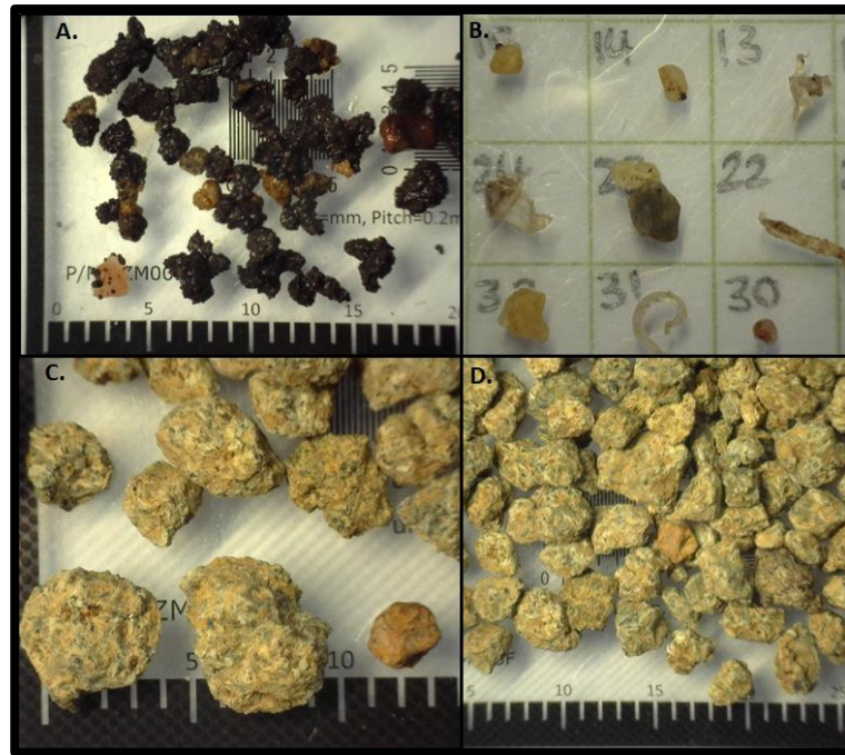
Figure 29: Close-up images of the volcanogenic unit. (A.) showing basalt and volcanic glass between 561 – 581 cm, (B.) showing volcanic glass between 581 – 601 cm, (C. and D.) showing close-ups of the K-feldspars and the transition to non-basaltic volcanic material located at the bottom of the core between 680 – 699 cm. Sclae A, C and D in mm. Pannel B scale in cm.
