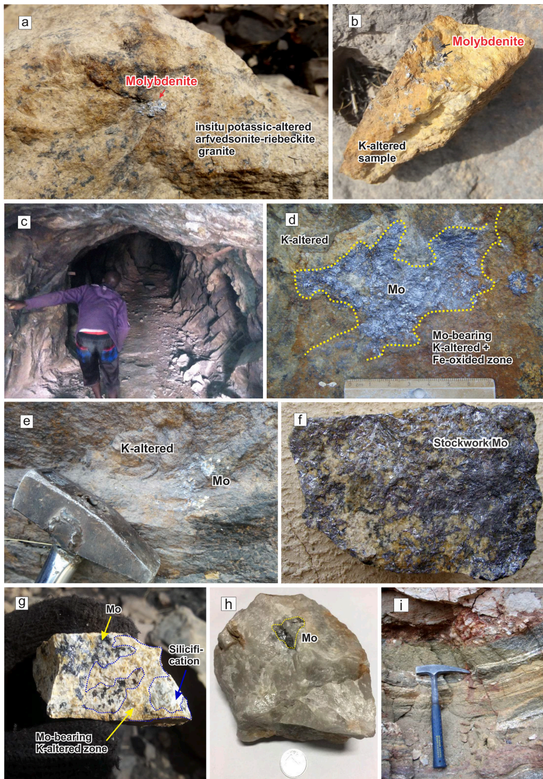
Fig. 7. Mo-Sn mineralization styles in Kigom complex (a) Molybdenite-bearing arfvedsonite-riebeckite granite outcrop; (b) Disseminated molybdenite in K-altered arfvedsonite-riebeckite granite; (c) Abandoned mine shaft in the Kigom complex. (d) Vertical profile of arfvedsonite-riebeckite granite showing K-altered zones, a molybdenite-rich layer, and Fe-oxide overprinting; (e) Localized disseminated molybdenite patches; (f) Stockwork molybdenite veinlets; (g) Patchy molybdenite in silicified K-altered granite; (h) Molybdenite associated with quartz crystals; (i) Cassiterite-bearing gravel layer in alluvial deposits west of Terema.
