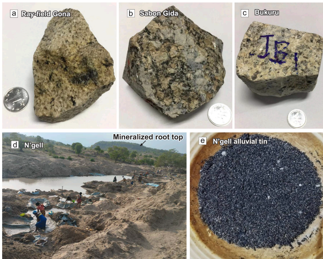
Fig. 4. (a-c) Hand specimen photographs of: (a) Rayfield hornblende-biotite granite, (b) Sabon Gida biotite granite, and (c) Bukuru biotite granite. (d) Field photograph of alluvial tin-columbite mining operations in N'gell, Jos-Bukuru Complex, showing the mineralized biotite granite pluton (foreground) with weathered roof zones that sourced the detrital tin and columbite now concentrated in adjacent river channels. (e) Recovered columbite concentrates from the N'gell alluvial site.
