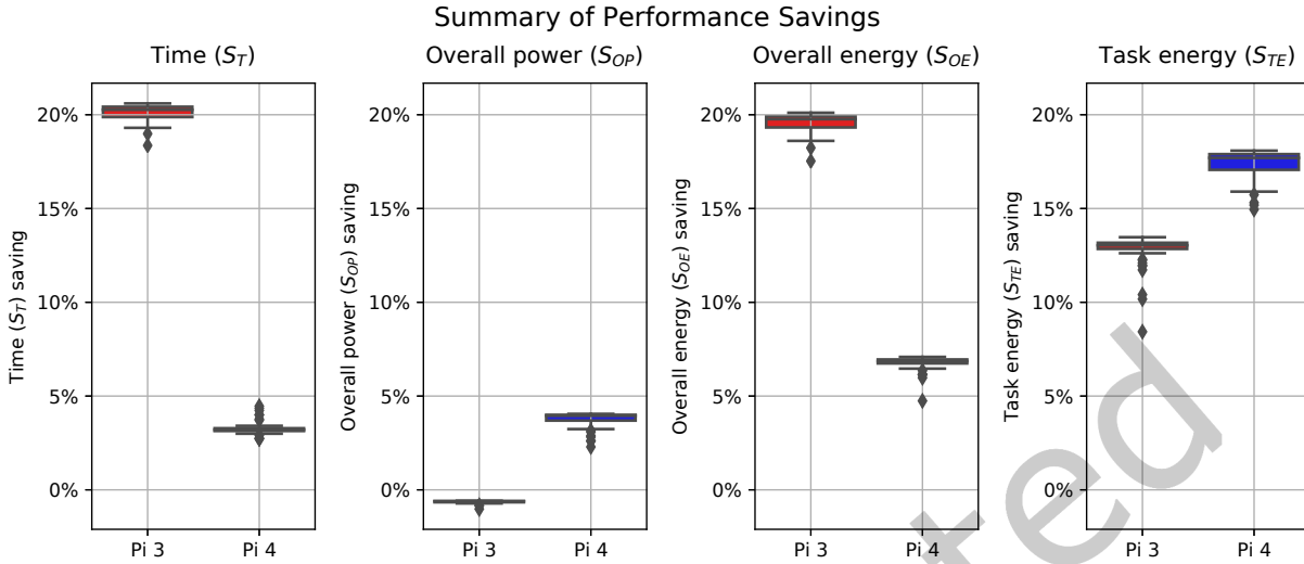
Fig. 12. Summary of best performance savings in time and energy on each platform. The y values represent the mean performance saving for each criterion ( S_T , S_{OP} , S_{OE} and S_{TE} ) for each specific sensor and measurement count. These savings are as defined in Eqs. (2), (6), (4), and (9). For each combination of sensor count ( S ) and measurement count ( M ), the mean performance gain across SVM feature counts > 1024 is collated. This set is shown in the box plot: the box contains the quartiles and the whiskers extend to show the rest of the range, with the exception of outliers, which are shown as dots. (The negative value for S_{OP} on the Pi 3 indicates that the modified algorithm had a net cost - more power was required by the modified coroutine execution pattern than by the unmodified sequential execution pattern.)
