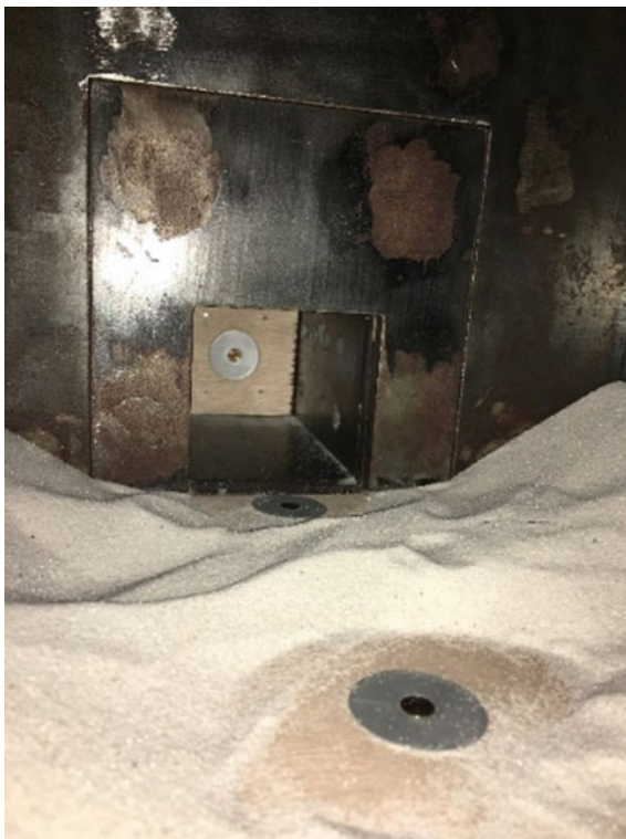
Fig. 1.14 Inside view of the model stope and locations of soil pressure sensors
