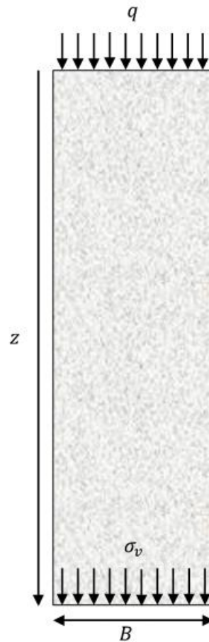
Figure 5.6. Fill in a square stope subjected to surcharge pressure
