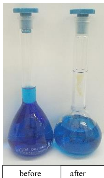
Plate 4.5: Colour of Acetonitrile Solution of Methylene blue, Before and After 24 Hours of Irradiation
