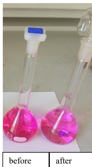
Plate 4.3: Colour of Isopropyl Alcohol Solution of RB, Before and After 24 Hours of Irradiation
