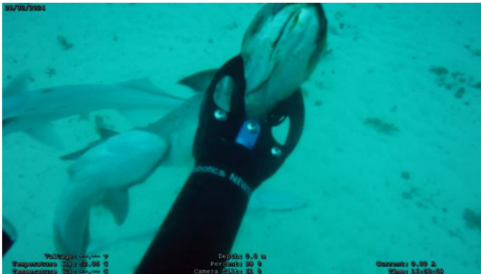
Figure 4.7. View from the pilot camera of the ROV. Mechanical arm extended forward carrying a mullet bait.
