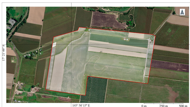
Fig. 1. High resolution RGB (Red, Green, Blue - visible spectrum) drone orthomosaic image reveals the location of palaeochannels close to ground surface. The drone image (outlined with a red line and in lighter shade) is superimposed onto satellite imagery obtained from the Global Mapper software (Source: Marcus Bulstrode, Queensland Government Department of Primary Industries).
