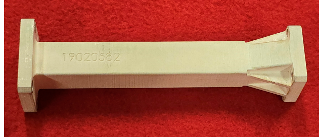
Figure 4. Additively manufactured polymer 100 mm polarizer from Swissto12 (AM Polymer 100 mm).
