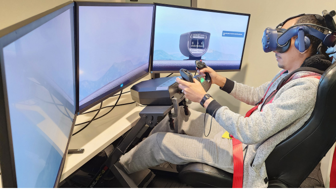
Fig. 2. Experiment set-up with attachment of HTC VIVE Pro Eye, and Equivalant EQ02 life monitor sensor belt and recording device. The experiment was performed using the Next Level Racing Motion Platform V3 (NLRMP V3).
