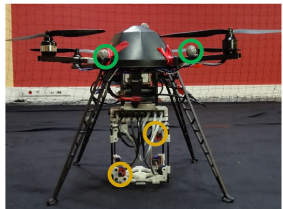
FIGURE 6. The MiKroKopter quadrotor UAV used for the DREGON dataset, with 3D printed 8-channel microphone array mounted on the bottom. Green circles highlight two of the passive markers used for motion capture and yellow circles highlight two of the microphones (best seen in colours). Copyright ©2017 IEEE [21].
