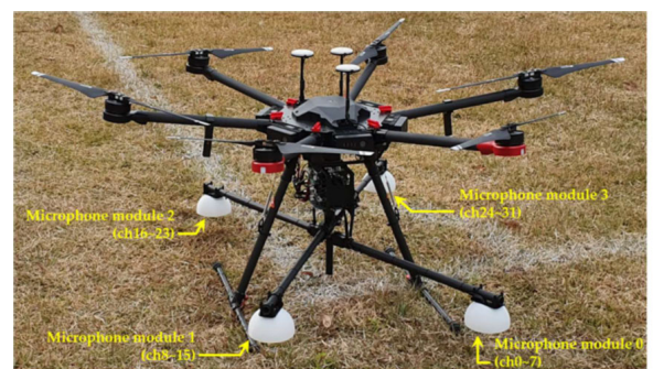
FIGURE 7. Four microphone modules, each with eight MEMS microphones, as shown in Figure 13 [28].
