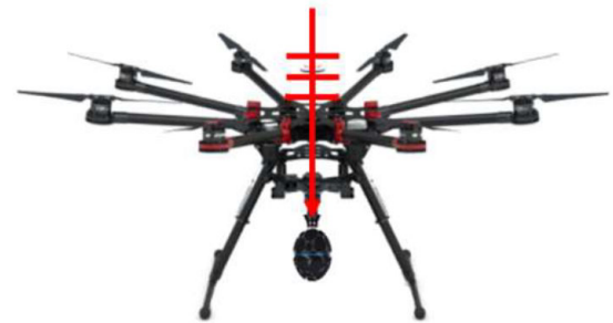
FIGURE 12. ZM-1 Ambisonics with 19 MEMS. The red arrow indicates the position of the microphone. Copyright ©2021 IEEE [48].
