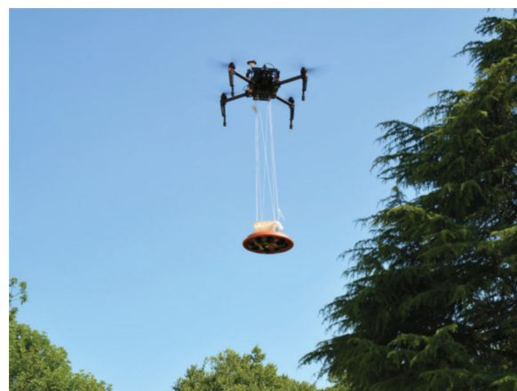
FIGURE 16. Circular microphone array mounted on the bottom of the Matrice 100 quadcopter, through a set of four nylon cords of 1 m length each. Copyright ©2020 IEEE [19].
