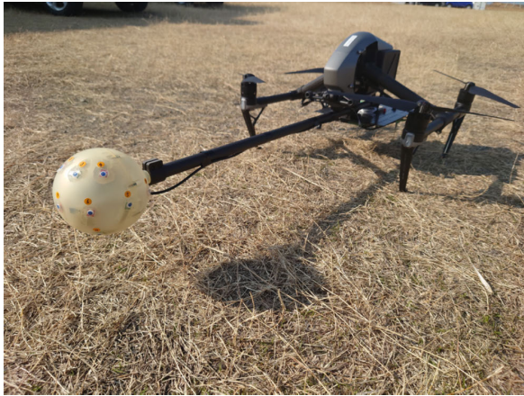
FIGURE 17. DJI Inspire 2 drone and 16-channel microphone array on one side of the drone. The distance between the drone centre and the microphone array is 50 centimetres [34].
