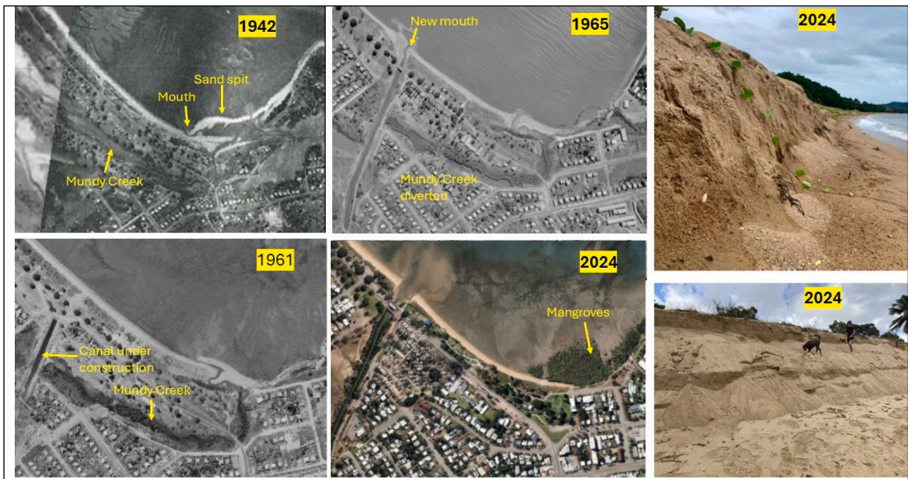
Fig. 3. Historical aerial images of Mundy Creek from 1942 to 2024; photographs of (top right) the 2 m high sand cliff with no beach before beach nourishment and (bottom right) 2 weeks after beach nourishment, showing toe erosion at the bottom and slumping on top. Photos courtesy of the Queensland Government, Bruce Muller and EW.
