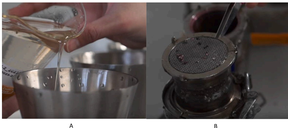
Fig. 7. Images of sample filtration using the size classed filtration system, A) demonstrating the decanting of the sample into the funnel, and B) particulates trapped on one of the stainless-steel filter discs.
