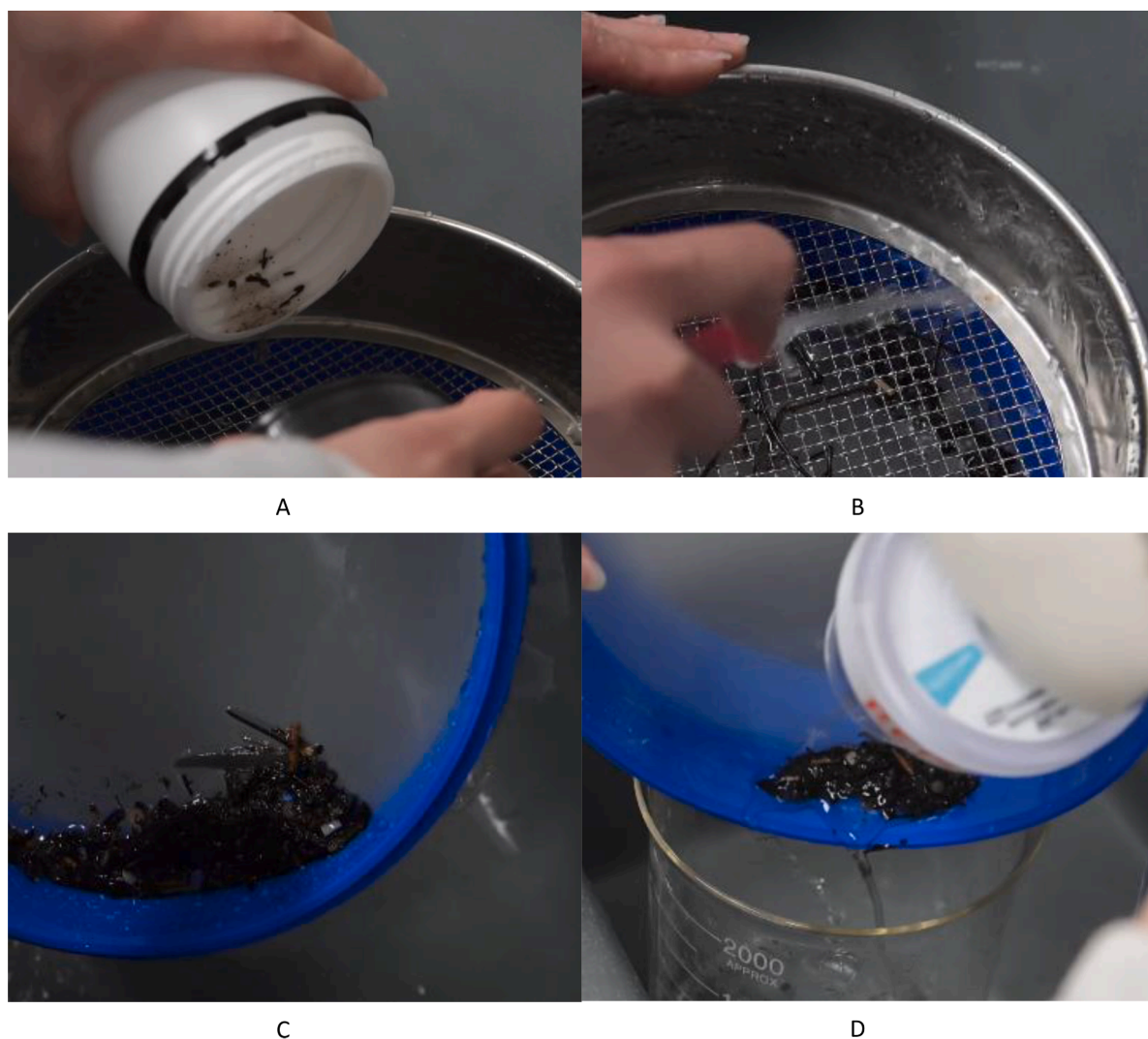
Fig. 3. Images of the sieving process. A) the sample being poured over the stacked sieves; B) triple rinsing the sample jar contents over the sieve; C) digestate contents concentrated into the corner of the 0.2 mm sieve; and D) transfer of the digestate into a 2 L glass beaker (400 mL maximum).
