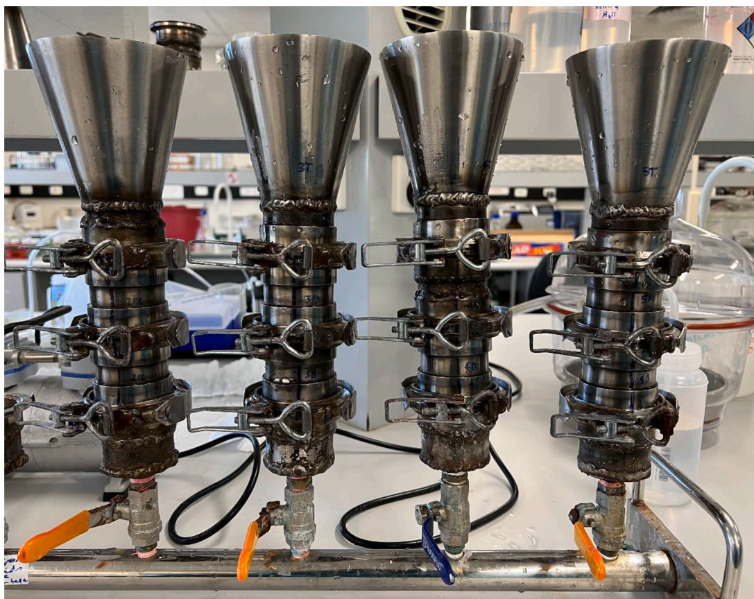
Fig. 5. Size classed filtration system adapted from Schlawinsky, Santana [17]. The system is comprised of a series of stainless-steel expanders that act as stacked sieves, attached to a vacuum manifold. The use of a vacuum manifold allows for multiple stacks to be used simultaneously (four stacks shown here), whilst providing a stable base. The ball valves allow the stacks to be individually drained when open, or to soak in Nile Red (NR) stain when closed. Stainless steel materials were used to reduce corrosion and the potential of extraneous contamination of the samples.
