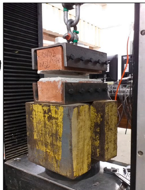
Fig. 8. Isometric and as-constructed image of apparatus for direct tension on unit-mortar interface; image captured after failure of joint.
