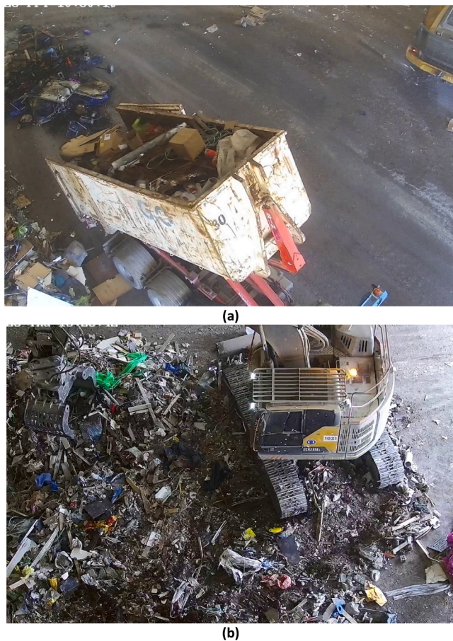
Fig. 1. Real world example of CDW waste. (a) an example of a typical mixed CDW-containing skip bin. (b) Pile waste being spread and examined with an excavator.
