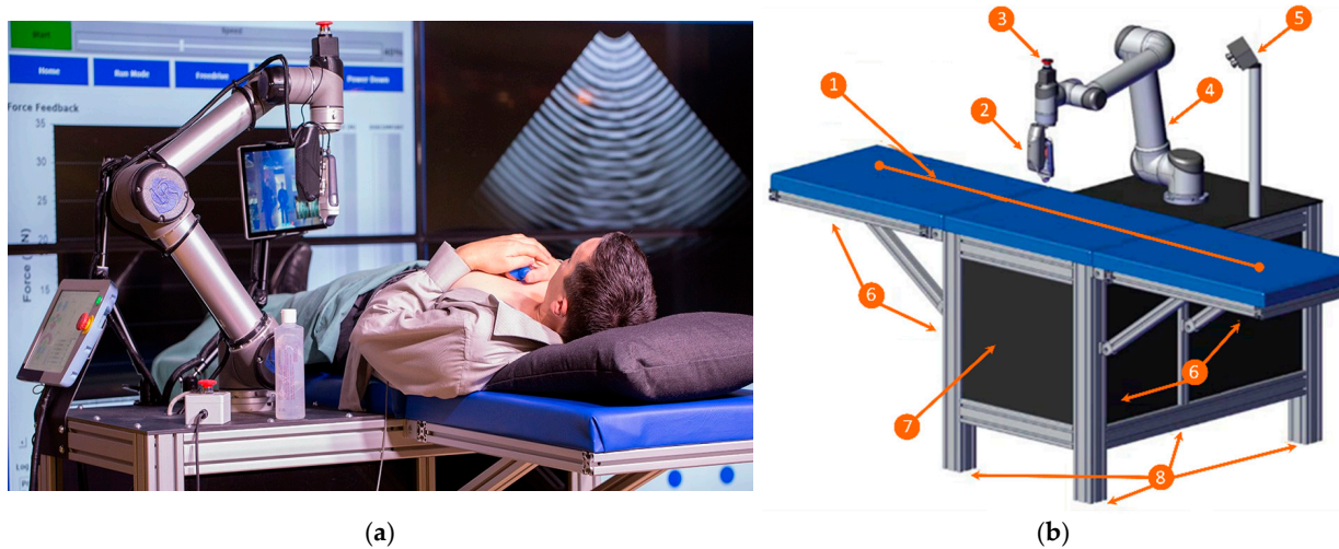
Figure 2. (a) Haptically-Enabled Robotic Ultrasound Platform; (b) CAD model of the HaptiScan platform.
