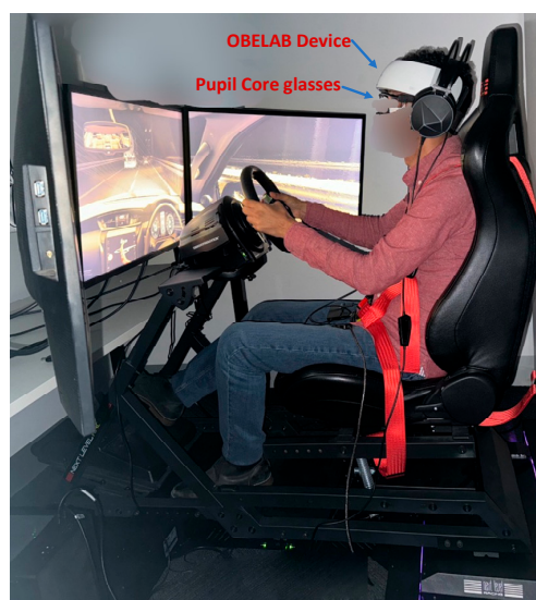
Figure 1. Driving simulator setup designed to replicate real-world vehicle dynamics and driving conditions using motion platforms and responsive control hardware.
