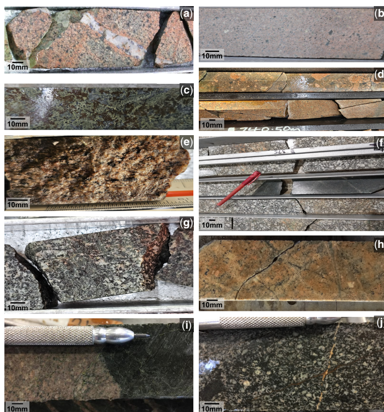
Fig. 3. Photomontage of intrusive and host rocks from Macquarie Arc deposits. (a) Trundle Park TD002 420.10–420.13 m. Monzonite porphyry with quartz–calcite–molybdenite vein. Dated by Re–Os method. (b) Northparkes E22D248. Hematite dusted 'red rock' alteration of partly brecciated quartz monzonite. (c) PC179 Cadia Quarry. Garnet–epidote skarn after feldspathic, calcareous sandstone near quartz monzonite intrusion. (d) Drill hole Mordialloc prospect CTD006. Feldspar-rich quartz monzonite with mafic basaltic andesite dyke. (e) PC179 Cadia Quarry. Monzonite. (f) Mordialloc prospect ERE22D248. Quartz monzonite phase – associated with mineralization. Dated by U–Pb (zircon). (g) PC302 diorite from Cadia–White Engine. (h) EL48D58 Northparkes. Silicified and slightly brecciated monzonite. (i) Kaiser NKD003. Contact between the K-altered monzodiorite/diorite intrusion and the host andesite. (j) Kaiser NKD003. Typical biotite-altered porphyritic diorite to monzodiorite comprised of plagioclase, hornblende and minor quartz. Source: photographers: David Forster, Phillip Blevin and Joel Fitzherbert.
