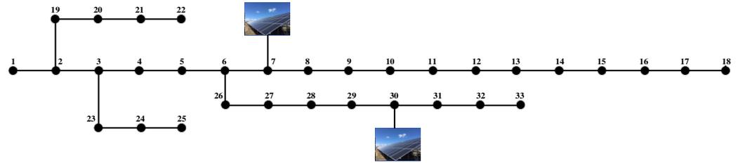
Figure 3. Simulated distribution network of IEEE 33 node.
