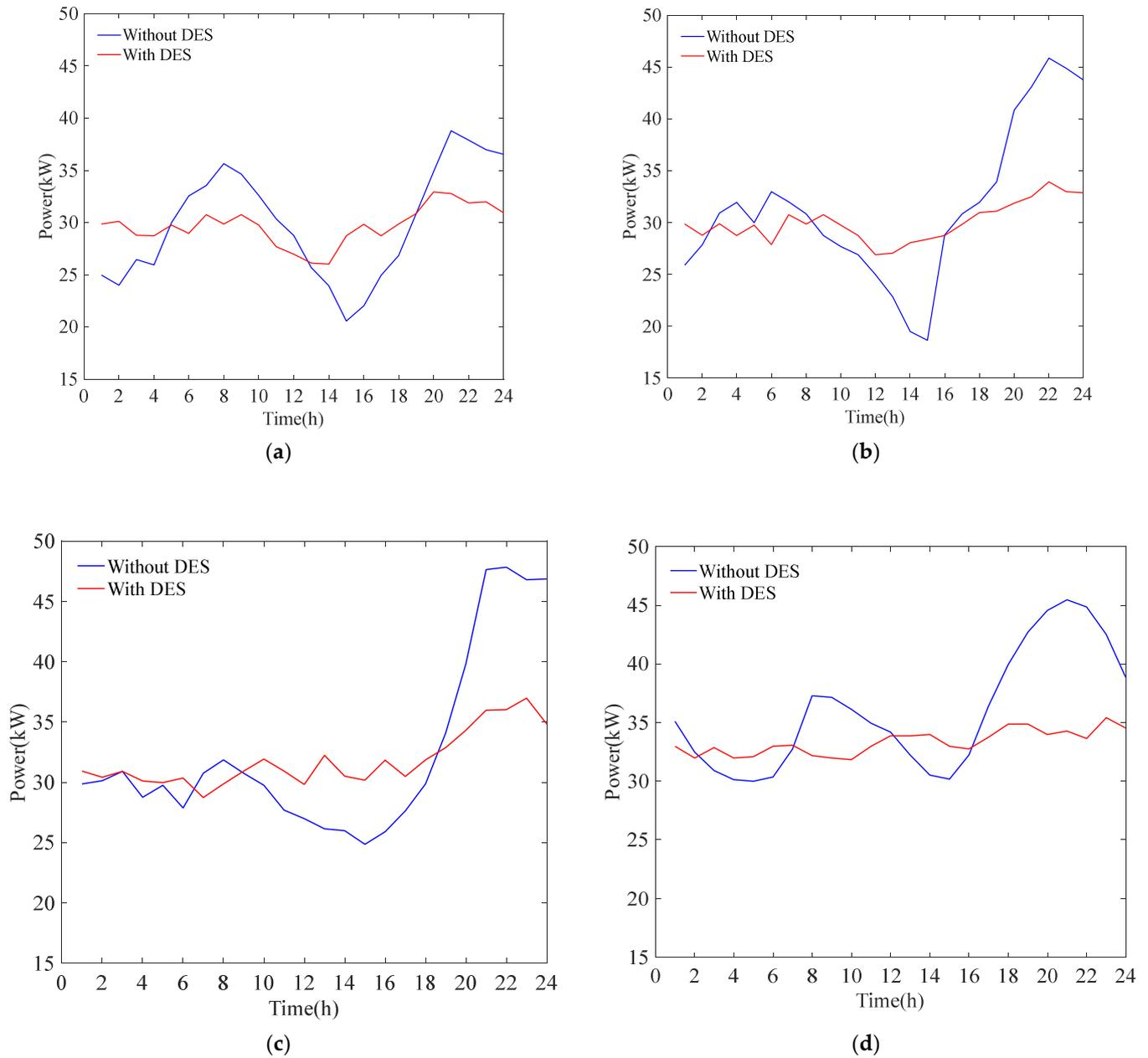
**Figure 5.** Daily net load profiles for MSCLSI-based simulated networks with and without DES: (a) spring, (b) summer, (c) autumn, (d) winter.
