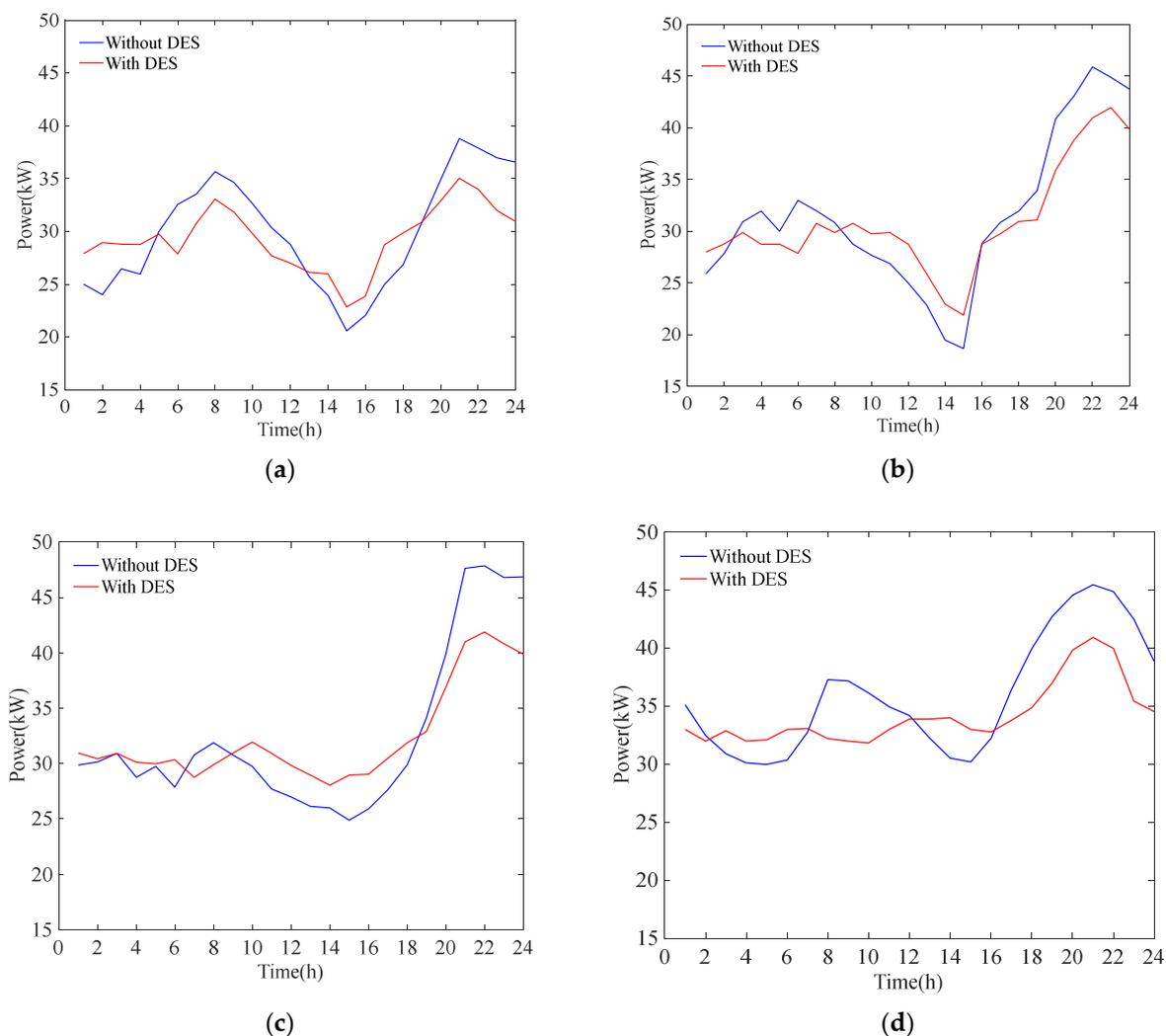
**Figure 7.** Daily net load profiles for CLSI-based simulated networks with and without DES: (a) spring, (b) summer, (c) autumn, (d) winter.
