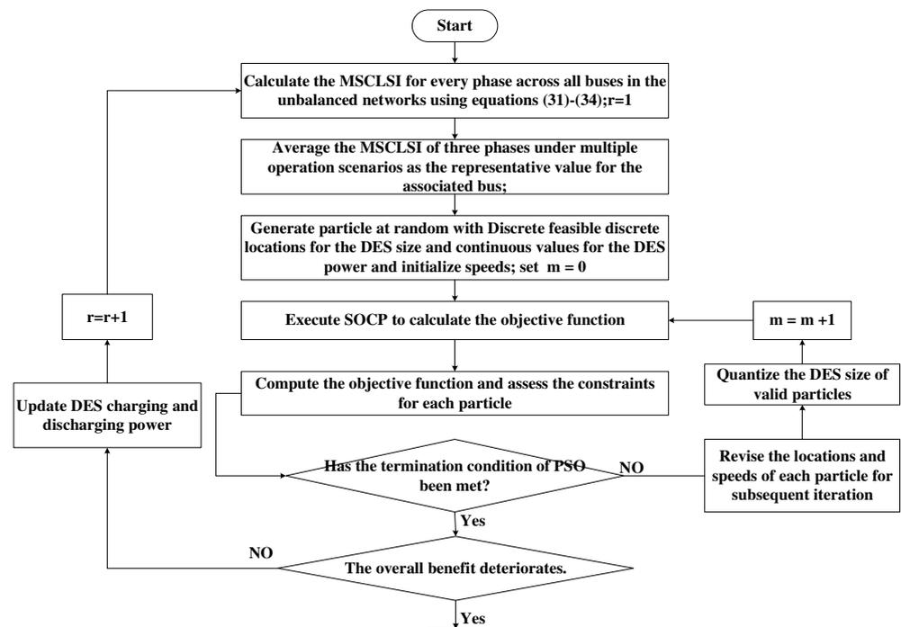
Figure 2. Flowchart of DES Sequential Placement based on MSCLSI.
