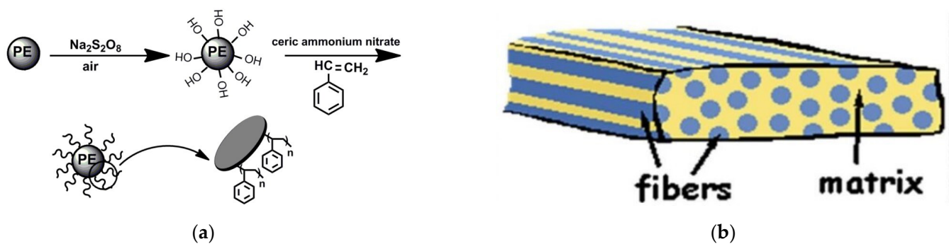
Figure 6. Schematic diagram of (a) polystyrene on UHMWPE powder [116] and (b) schematic diagram of FRPs [110].
