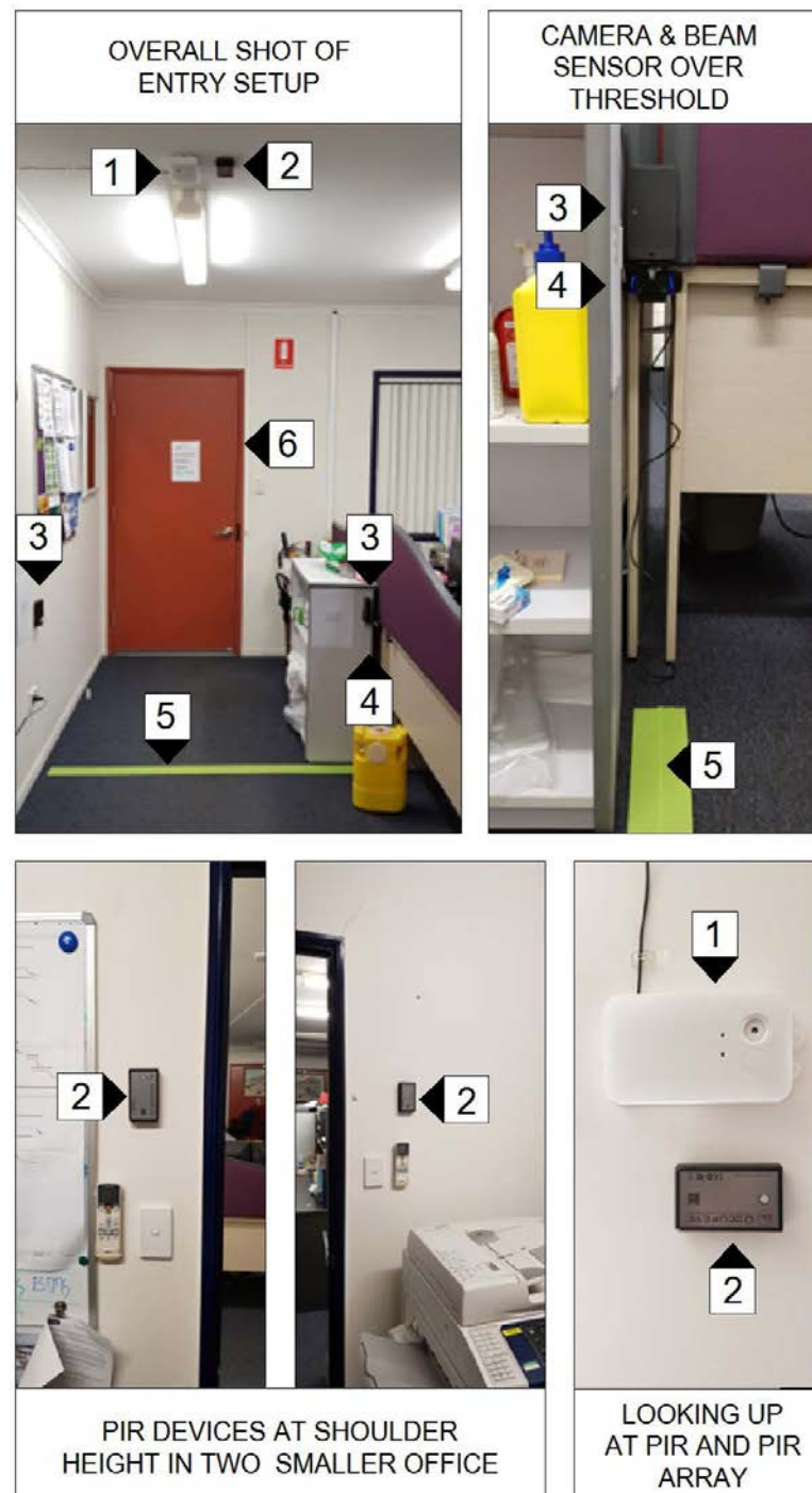
Figure 13 – Three sensor calibration activity layout (1: PIR array, 2: PIR, 3: Thermal beam) trialled for accuracy against a video camera (4) along a defined threshold (5) at the entrance (6) to a 3-room, non-clinical suite.
