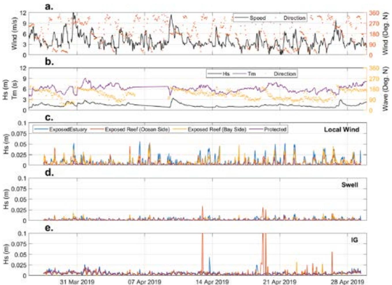
**Fig. 4.** Wind speed and direction (a), offshore significant wave height ( $H_s$ ) and direction (b), wave height for local wind waves (c), swell waves (d) and infragravity waves (e) at Port Hacking (27/03/2019–26/04/2019). Locations: Exposed estuary/entrance (blue), exposed reef (ocean side) (orange), protected (purple) and exposed (bay side) (yellow). (For interpretation of the references to colour in this figure legend, the reader is referred to the web version of this article.)
