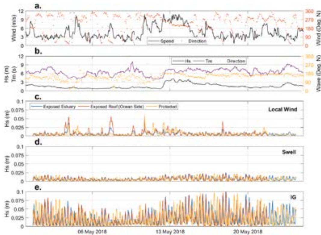
**Fig. 3.** Wind speed and direction (a), offshore significant wave height ( $H_s$ ) and direction (b), wave height for local wind waves (c), swell waves (d) and infragravity waves (e) at Gamay (30/04/2018–24/05/2018). Locations: Exposed estuary/entrance (blue), exposed reef, ocean side (red) and protected (yellow). (For interpretation of the references to colour in this figure legend, the reader is referred to the web version of this article.)
