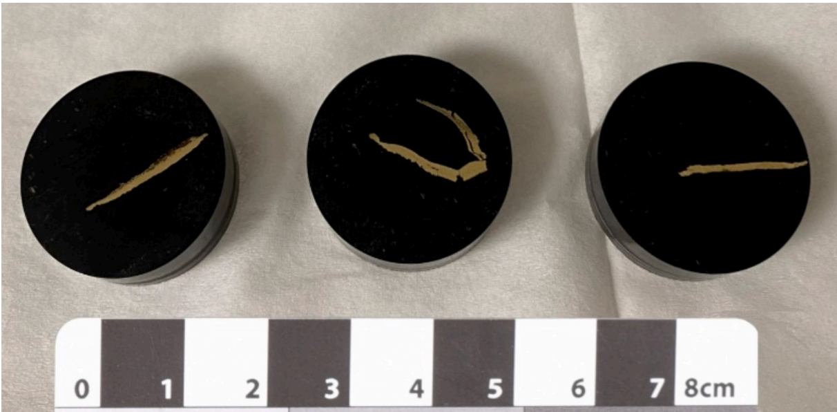
Fig. 3. Kenn Reef ships' hull sheathing samples embedded in black-coloured resin mount after polishing. Photograph by W. van Duivenvoorde.
