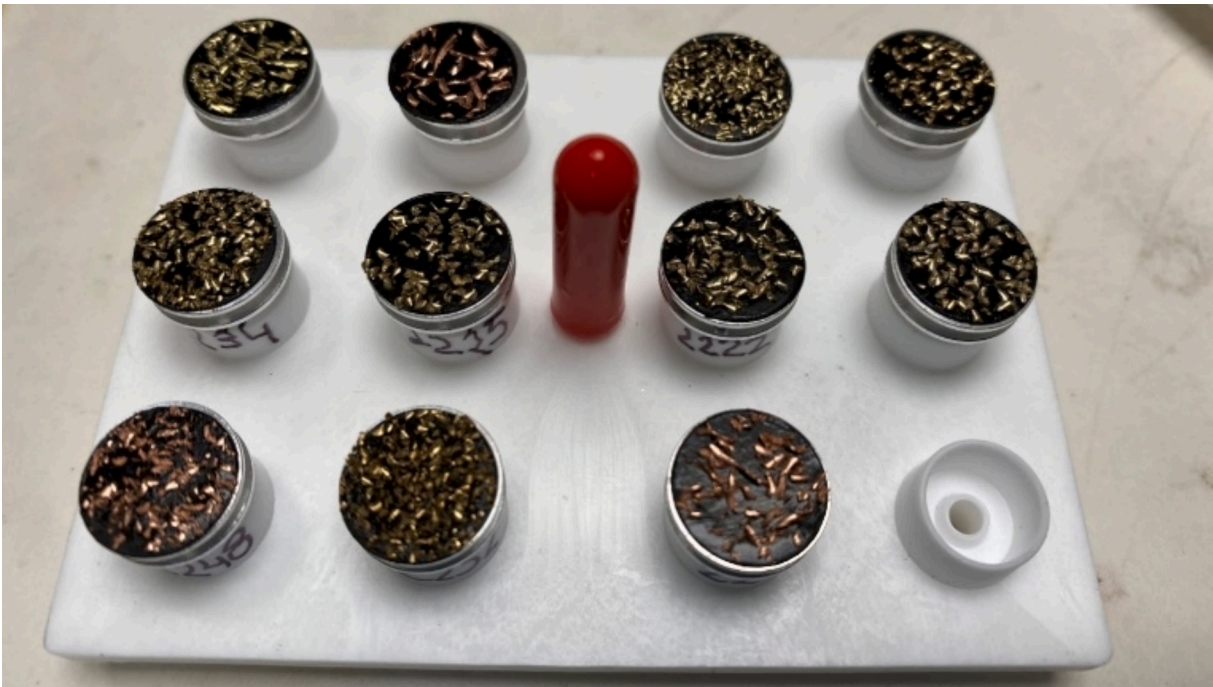
Fig. 4. Kenn Reef drill shavings mounted on aluminium stubs with carbon tape. Photograph by W. van Duivenvoorde.
