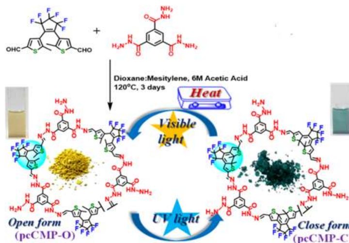
Figure 2.13: Synthetic scheme for the pcCMP and color changes in photo-isomers. [107]
