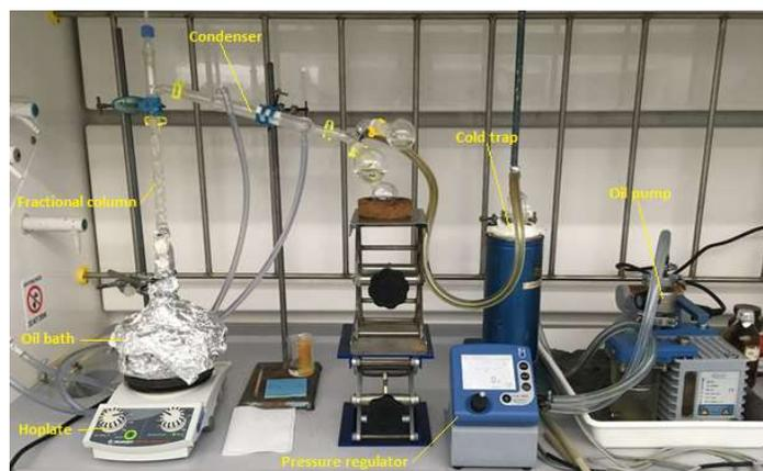
**Figure 3.61:** Fractional vacuum distillation setup.
