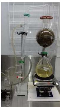
**Figure 3.20:** Glass-based steam distillation setup.
