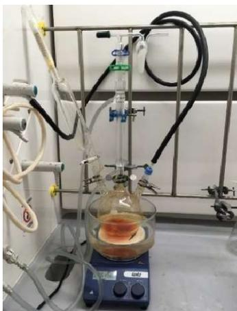
**Figure 3.71:** Reaction setup for the exhaustive methylation of acylphloroglucinols.
