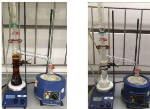
**Figure 3.22:** Liquid-liquid extraction using boiler (left) and distilled boiler water (right).
