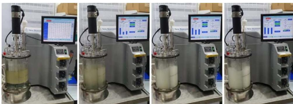
**Figure 3.46:** Initial LSG oil-water layers and generation of a stable emulsion.
