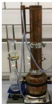
**Figure 3.21:** Copper-based steam distillation setup.
