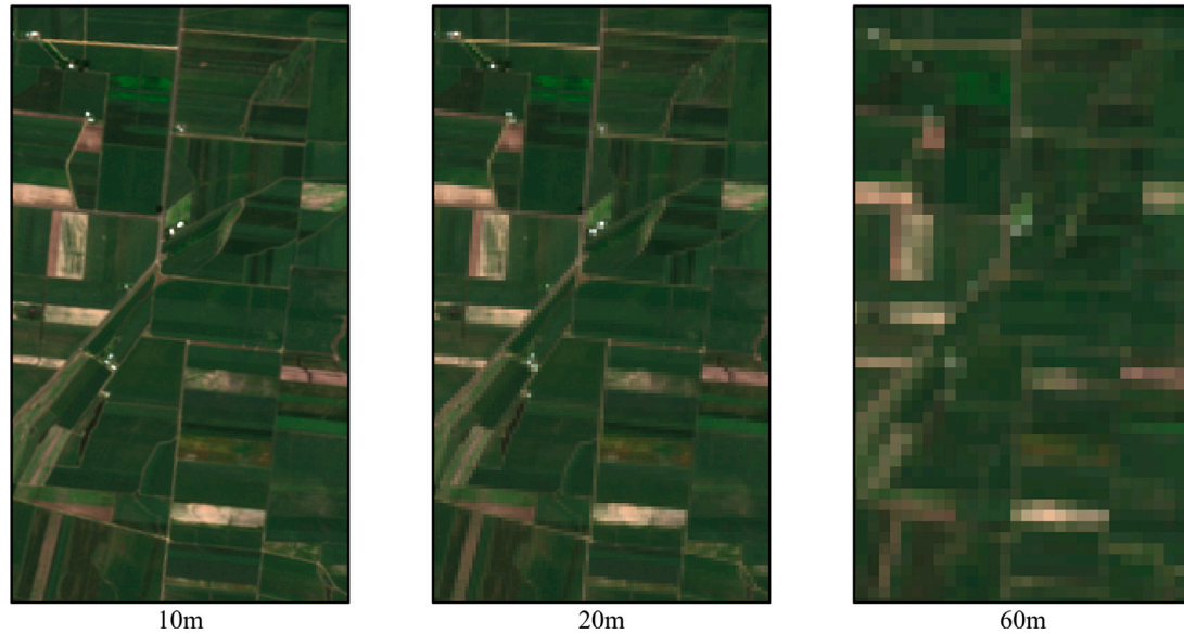
Fig. 2. Spatial resolution comparison of available Sentinel-2 resolutions. Sentinel-2 offers four bands at 10 m resolution, ten bands at 20 m resolution and twelve bands at 60 m resolution.
