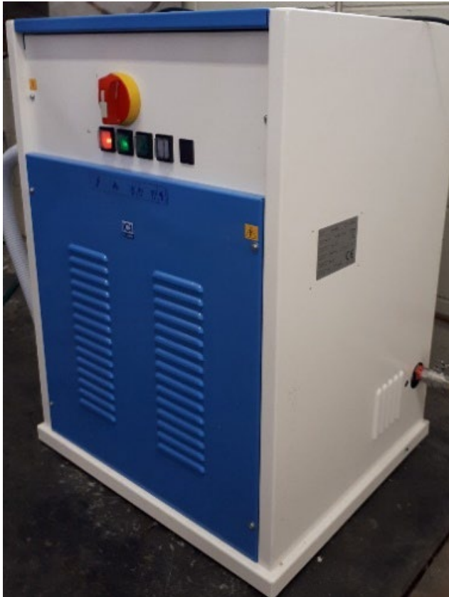
Figure 3-3: Maxi24 Ghindi Benvenuto steam generator.
