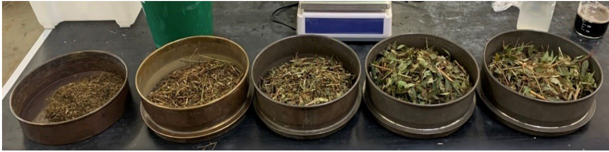
Figure 5-1: Laboratory Classification Sieves with Biomass Separated into Representative Size After Sieve Analysis.
