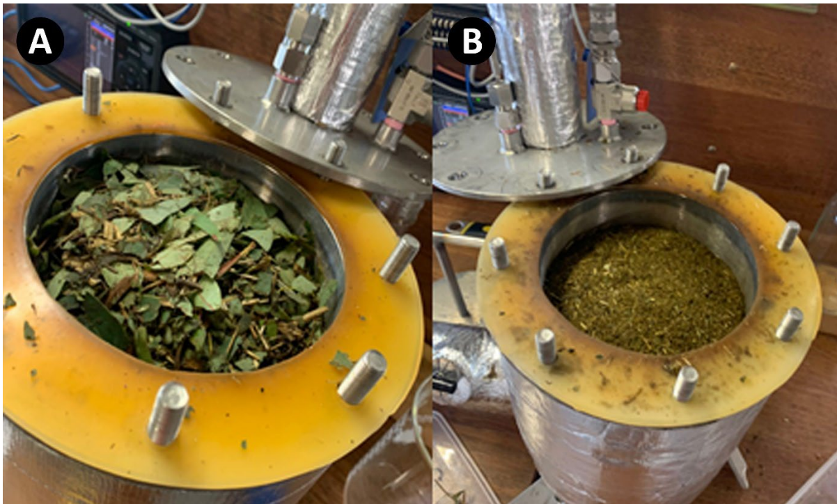
Figure 5-2: Biomass packing in distillation chamber. A) Uncut biomass, B) High reduction biomass.
