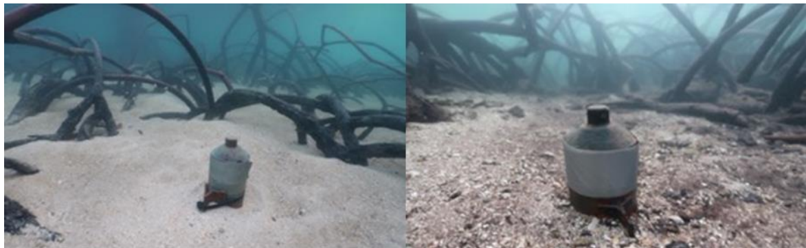
Fig. 4.2 Receivers deployed among mangrove roots.
