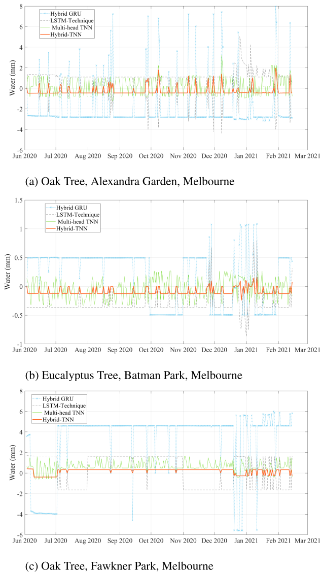
FIGURE 8. Comparison of irrigation water balance by Hybrid GRU [27] (blue semicolon line with x marker), LSTM-Technique [32] (grey dashed line), (3) Multi-head TNN [25] (green line) and (4) Hybrid TNN (red line) at (a) Alexandra Garden, (b) Batman Park, and (c) Fawknor Park. The hybrid TNN line is closer to zero (most optimum irrigation) than the other models.
