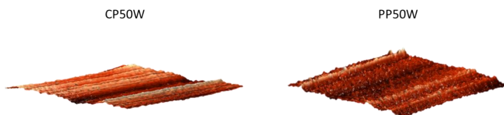
Figure S. 2. AFM scans of 3x3 μm of PP-OSMs samples after submerged in MiliQ water.
