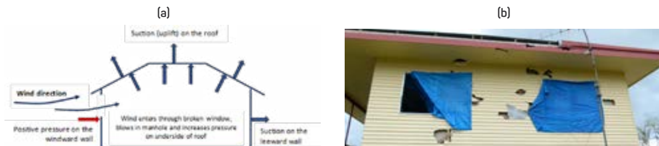
Figure 2: (a) Wind pressures on building and (b) example of damage caused by debris during a Tropical Cyclone Yasi.
