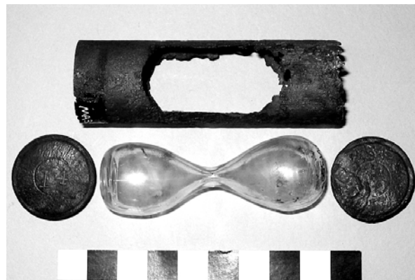
Figure 2 Disassembled 14 Second Sandglass
