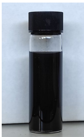
Fig. S 1: 600 W graphene solution in ethanol, ultra-sonicated for 5 minutes
