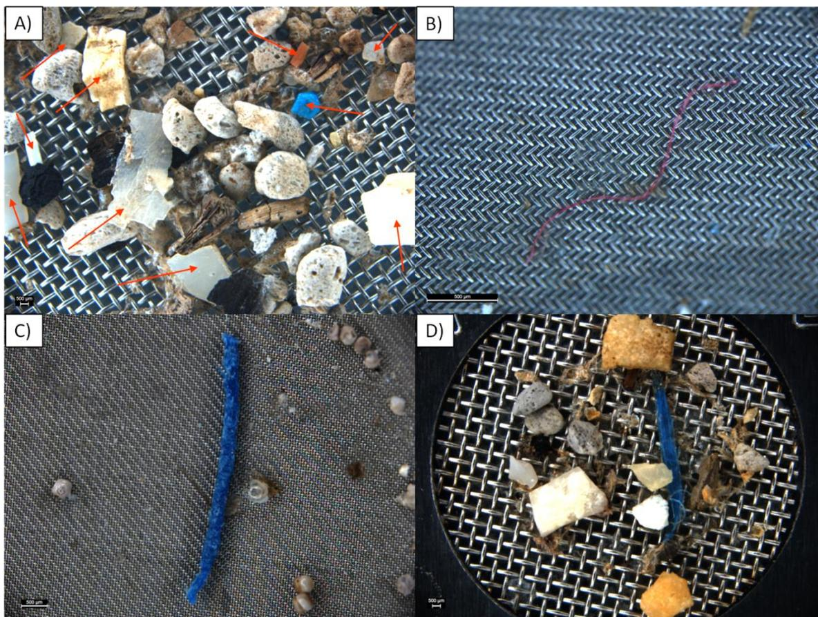
Figure A5.1 Plastic items isolated from surface seawater tows collected at the SS Yongala NRS in (a) April 2017, (b) June 2017, (c) May 2018, and (d) February 2019. Scale bars are representative of 500  $\mu\text{m}$ .
