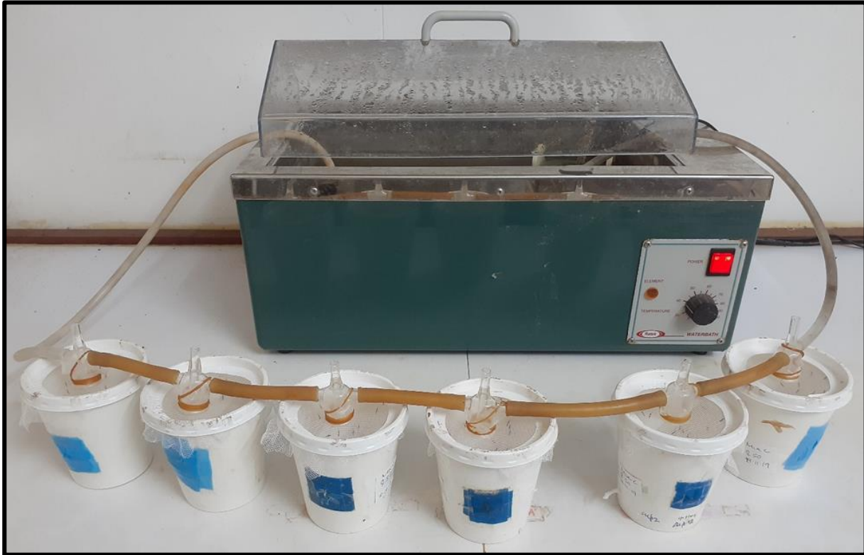
Figure 3.2. Direct membrane feeding assay (DMFA) set up. Cups connected in a series by tubes to a mini aquarium pump within the water bath which is maintained at ~38 °C.
