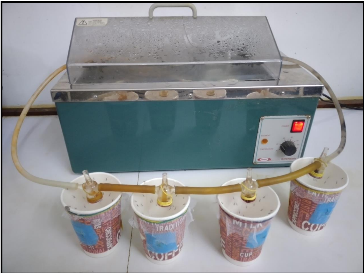
Figure 2.1. Direct membrane feeding assay (DMFA) set up. Cups connected in a series by tubes to a mini aquarium pump within the water bath which is maintained at ~38 °C.
