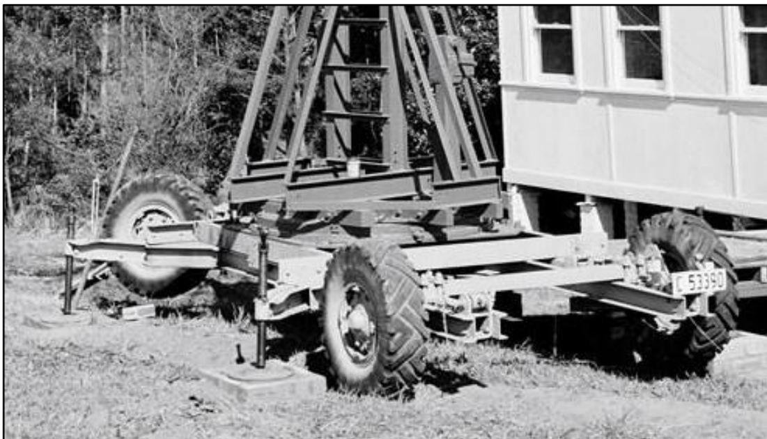
Figure 210: The ex-British Army gun-laying 200 MHz radar trailer which was used for the alt-azimuth mounting for the Murraybank 21-ft aerial (Adapted from ATNF Historical Photographic Archive: B3973-1 Image Date: 18 May 1956).
