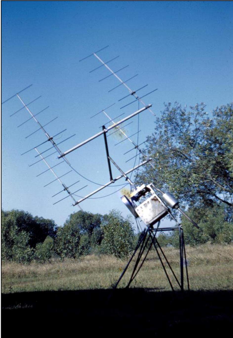
Figure 80: A four-element Yagi array at Potts Hill (Courtesy of ATNF Historical Photographic Archive: P12205-1)
