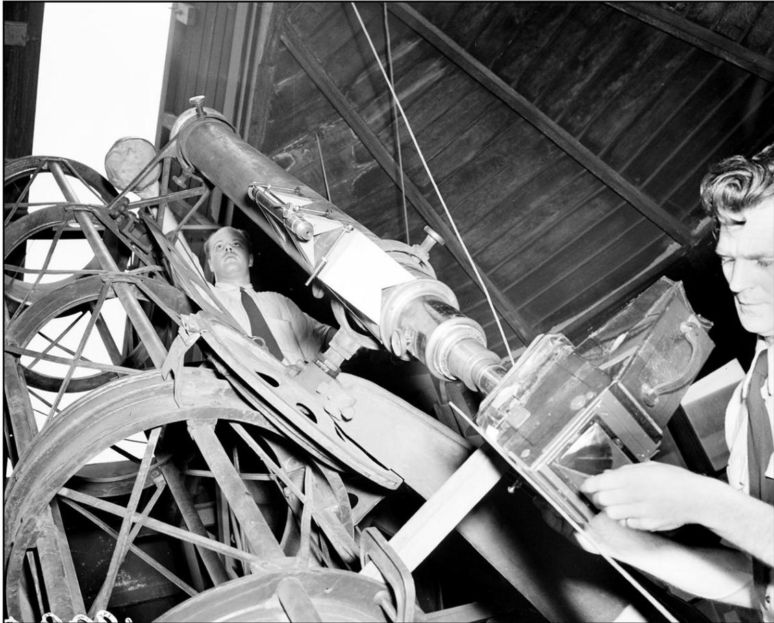
Figure 86: The Sydney Technical College telescope used for solar imaging during the eclipse observations. Photographs were taken using the 15 cm (6-in) guide-scope attached to the 46 cm (18-in) reflector (Courtesy of the ATNF Historic Photographic Archive: B1899-7).
