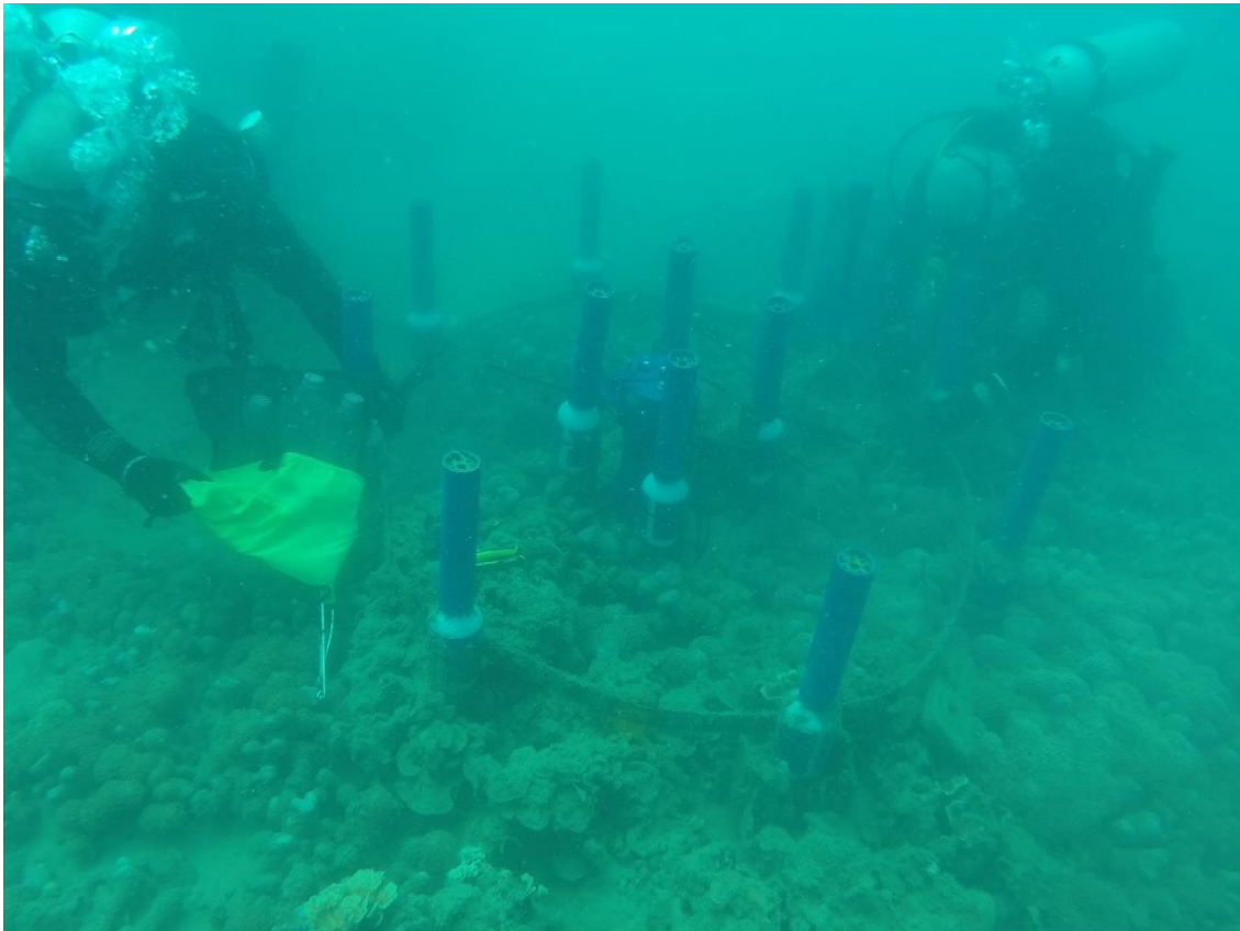
Figure 2.17. The sampling design set up for investigating the role of spacing on collection efficiency for sediment traps. In the centre is the standard NESP trap frame which is surrounded by the 9D spaced traps (Photo: Cassandra Thompson).
