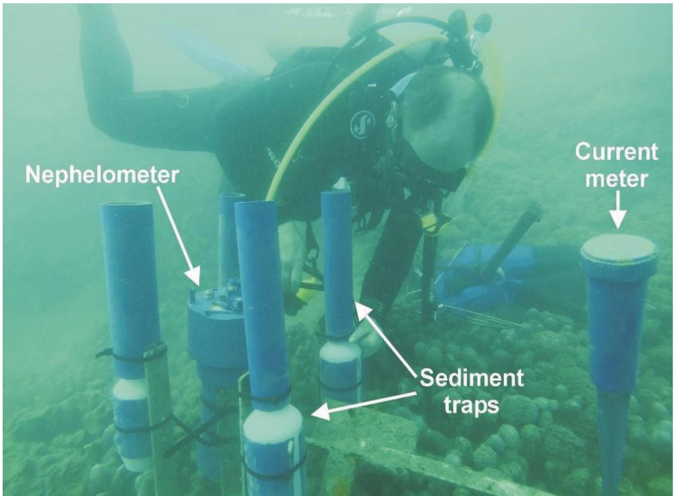
**Figure 3:** Typical instrument set up at the seven sites with nephelometer (turbidity, light and RMS pressure sensors), current meter and four replicated sediment traps (Image: Ian McLeod).
