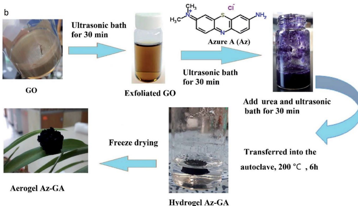
Figure 23. (a). Fabrication of the Try-Ni-MOF; (b). Az-via and a 3D GA are synthesized via a hydrothermal process; (a,b). Reproduced with permission, Royal Society of Chemistry [26]
