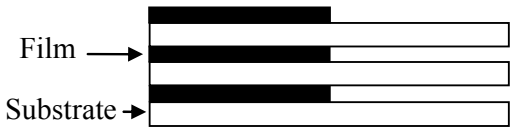
Figure 3: Cross section view of a number of substrates with film deposited on half of the surface area stacked together for measurement of the sample and of the reference.
