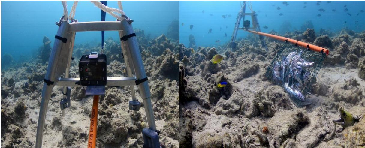
**Figure 3.1.** Baited remote underwater video survey (BRUVS) station deployed on seabed in reef habitat. BRUVS station comprises of a GoPro camera within an underwater housing on weighted metal frame, with a bait pole attached to attract predators, a current meter, and rope attached to surface float. Credit: Global FinPrint Project (<https://globalfinprint.org/>).
