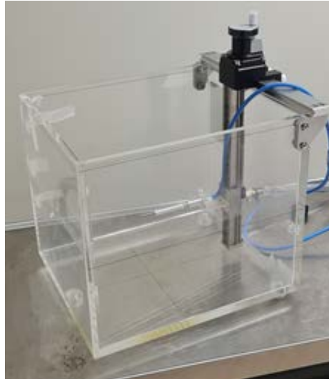
Figure 4.2: The PTW 1D water tank with Farmer chamber inserted
