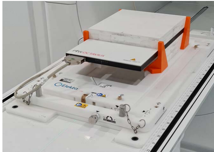
Figure 4.3: 1500 MR array setup for dose map measurements on the Elekta supplied QA Platform. The in-house developed 3D printed holders (orange) aid with positioning
