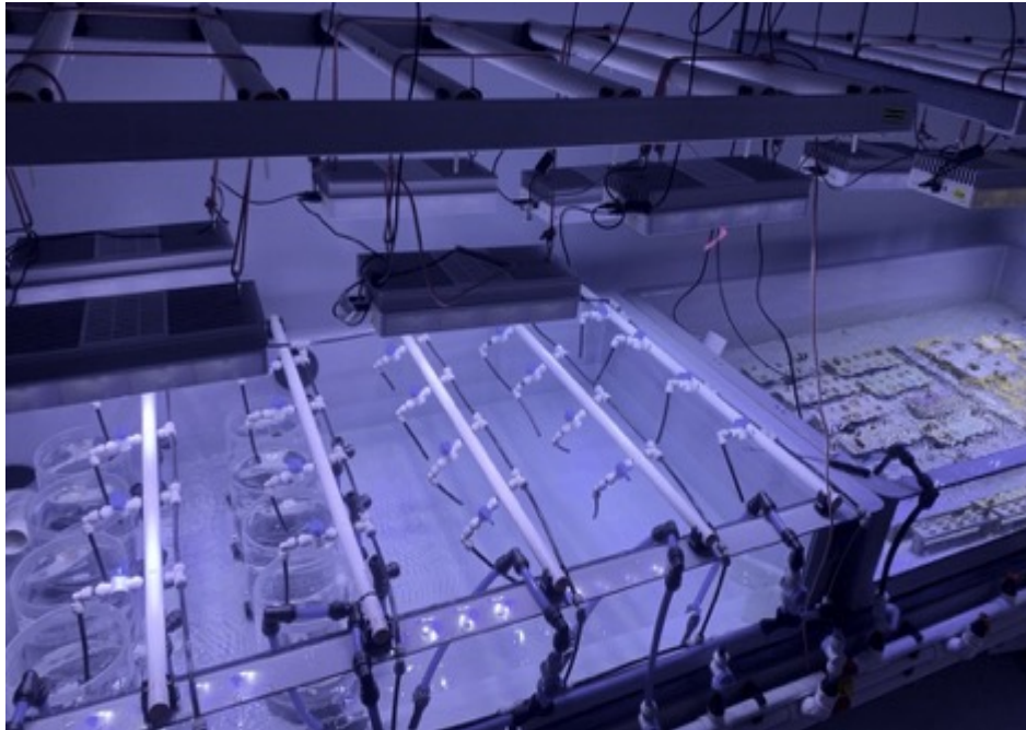
Figure 2.1 Tank set-up. (Left) Cylindrical feeding chambers, with coral plug trays, a magnetic stirrer, seawater inlet and outlets, were placed on water driven stir plates to homogenize prey in individual chambers. Overhead lights emulated day and night oscillations in light intensity on the reef where colonies were collected. (Right) A 250 L bath tank held fragmented corals on plug trays to acclimate to aquarium conditions.
