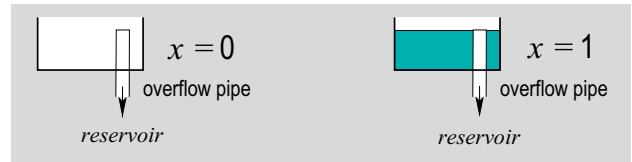
Fig. 7 Representation of logical values by a water tank
