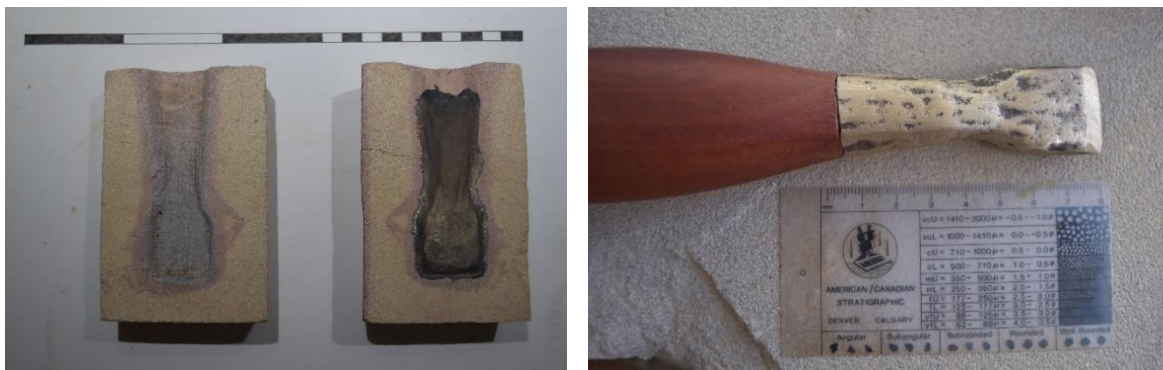
Figure 48. & Figure 49. Bronze chisel two-piece cast mould made from sandstone and finished bronze chisel
