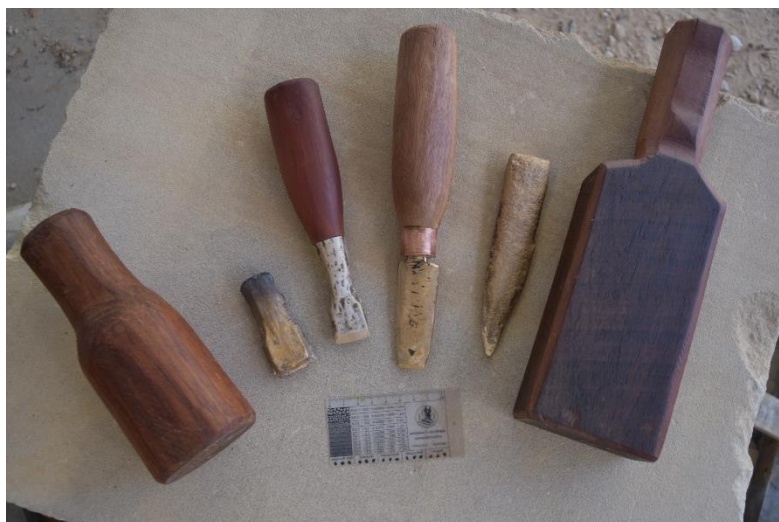
Figure 47. Bronze tool kit including three chisel forms
