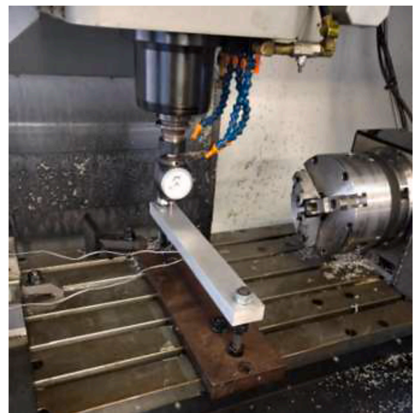
Fig. 2. Residual stress measurement apparatus.
