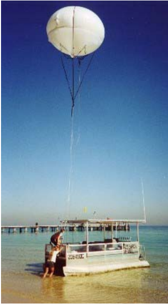
Figure 2.6 Blimp attached to the front end of the boat and kept at a height of approximately 10 m while towing during transit.
