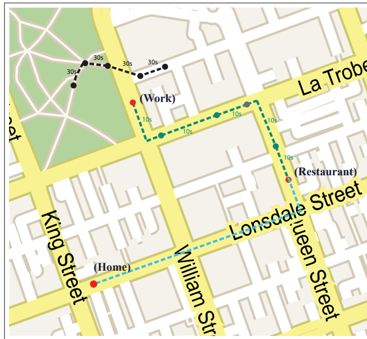
Fig. 4.1 Two trajectory segments with different sampling rates. Top left (black) is a walking trajectory with a sampling rate of 30 seconds and bottom right (green) is a driving trajectory with a sampling rate of 10 seconds. The grey dot represents a missing point which may result in a high-variance in the estimation of speed. The green trajectory shows a user stops at a restaurant after work, then goes home after after dinner; notice that the time intervals between work to restaurant and restaurant to home are different.
