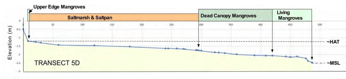
Figure 5.56. Profile of Transect 5D showing elevations measured in Oct 2018 and tidal wetland vegetation zones including canopy mangroves that died in late 2015.
