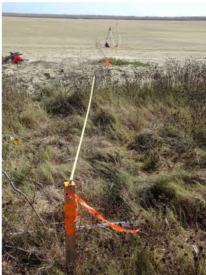
Figure 2.3. The 'head' of Transect 1A with measuring tape to the 30-metre mark (next to rotary laser on its tripod) showing the alignment towards the seaward mangrove fringe. Note the expansive saltpan – a common feature of these Gulf transects.
